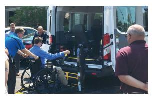
Drivers take turns using a wheelchair lift or ramp and learning the proper procedures for loading and securing a wheelchair passenger. Hands-on training helps to prepare drivers for real-life conditions they will encounter with actual passengers.
