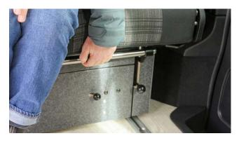
If the bench still moves, it is not locked into one of the three positions. Pull up on the bar again and continue to move until you feel and hear the seat click and lock into place.
