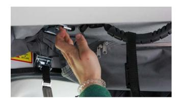
Turn and face the back of the van. Using the handles, push up on the roof (not the bed) with equal pressure on both sides. Guide the roof as far as your reach allows and then release. Then while holding the black strap, push up on the bed. Be sure to leave the black strap hanging as this will be helpful when lowering the bed. Both the pop top and bed are on hydraulics and will self extend when beyond your reach. Pushing the bed to the fully raised position will provide head room inside the van.
