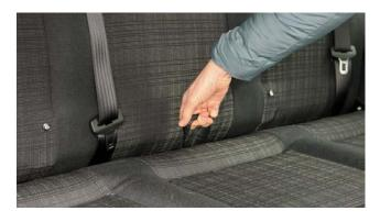
To fold down the back of the seat, find the black lever on the lower part of the bench frame on the driver's side and lift straight up (see photo on next page). This will release the backrest to fold down.
