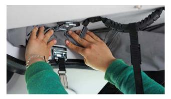
At this point, you'll be left with straps and a few billows of canvas hanging down. This will be hidden underneath the overhead interior cover. Roll up the fabric and tuck it behind the locking mechanisms. Then flip down the locking fastener.
