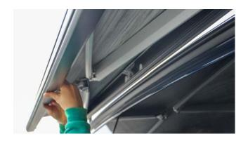
Slide each leg straight out ensuring the metal pin fully extends from the gray bracket joint before dropping the leg down to the ground.
