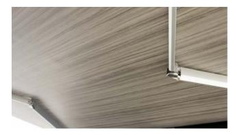
The awning should be taut with no slack. If it does have slack, retract the awning a bit until it is taut. Be sure to use the supplied awning stakes to secure your awning legs to the ground.
