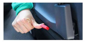
Swivel seat slowly towards the center of the van and adjust the seat sliding position as well as the seat back (to 90 degrees) accordingly. You may need to slide the seat forward and back a few times as you swivel it to clear obstacles. The seats do not lock when swiveled, but will lock when returned to a forward facing position.
