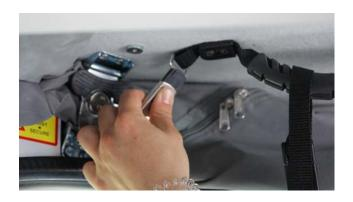
On that same side, flip down the black wing handle on the pop top bracket. You will turn this handle clockwise and counterclockwise to lock and unlock the bracket. To unlock the bracket, turn the black wing handle counterclockwise and release the top of the bracket hook from the bottom bracket bar.
