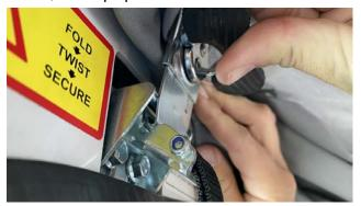
Close the click-lock mechanism by sliding plastic piece into metal. Perform this step on both sides.
