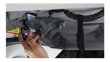
Secure the bracket to the magnet on the pop top. Perform these steps on the other side.
