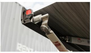
Once down, extend the leg to a level height and lock into place using the gray wing nut. This bracket joint is fragile and will break if the previous instructions are not followed.
