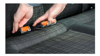
The two felt tabs on either side of the rear bench seat will then rotate to their original position.
