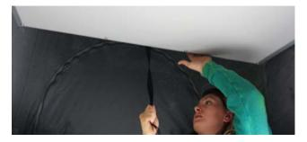
Pull down the bed by grabbing the black strap. It comes downs quickly in the last 6 inches so guide it. Before lowering the roof, make sure the pop top latches are held in place by the magnets.
