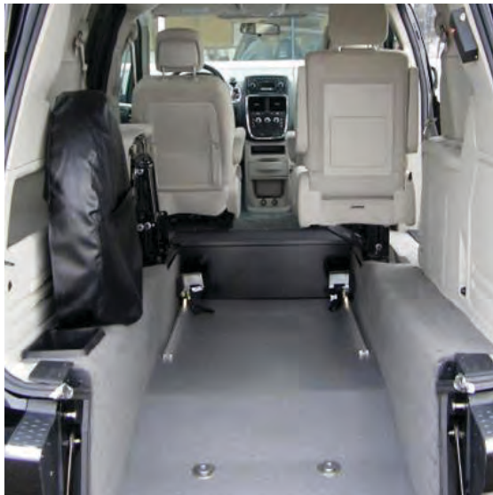
A full cut floor is shown with two 2nd row fold-out bucket seats. The 2nd row seat on the left is in its folded, stowed position.
