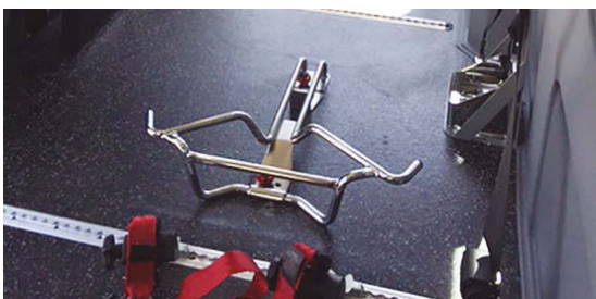
Floor mounts with antler design helps minimize effort required for loading and unloading.
