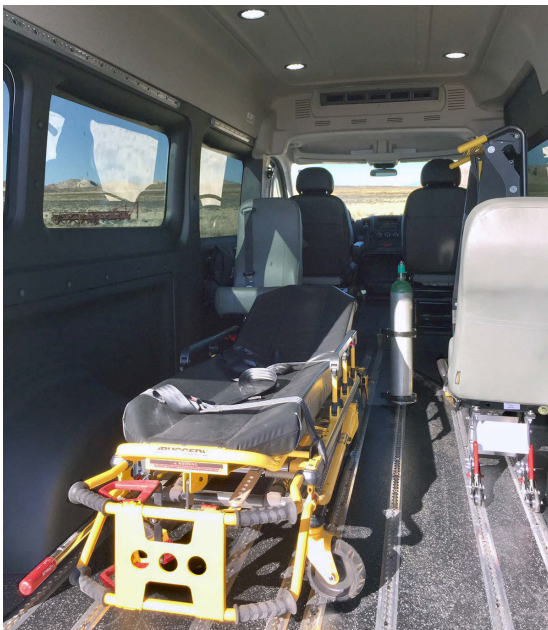
Wall mounts made of tough steel construction have an oversized rail clamp that keeps the cot stable.
