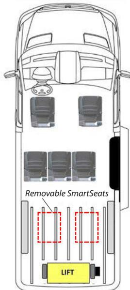
Rear access wheelchair lifts are available with 800 lb and 1,000 lb weight capacities. Additional SmartSeats with a removable base can be added to the rear section when not in use for wheelchair passengers.
