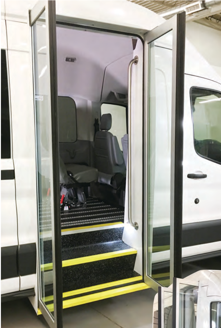
Built-in step lighting and entry stanchion pole is a standard bus door system feature.
