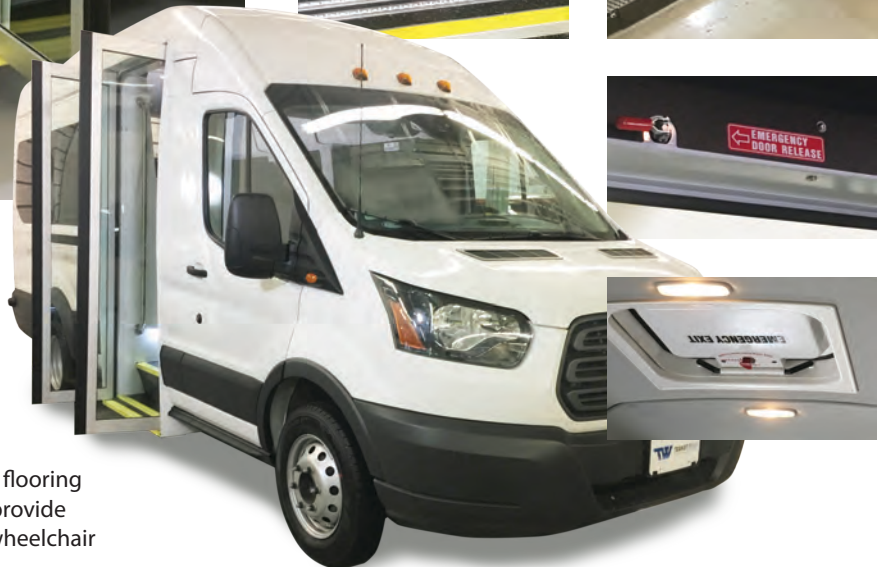
Built-in step lighting and entry stanchion pole is a standard bus door system feature.
