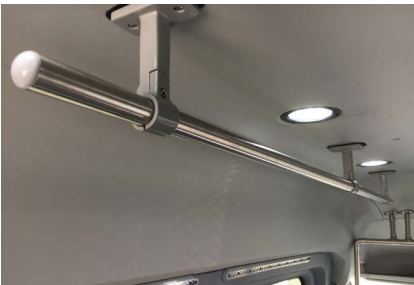
Ceiling mounted grab bar and overhead lighting.
