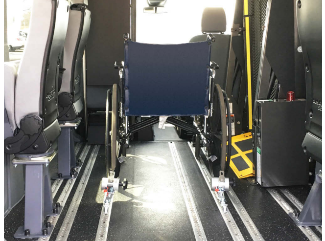
Extra-wide wheelchair shown in forward position secured to SmartFloor track.
