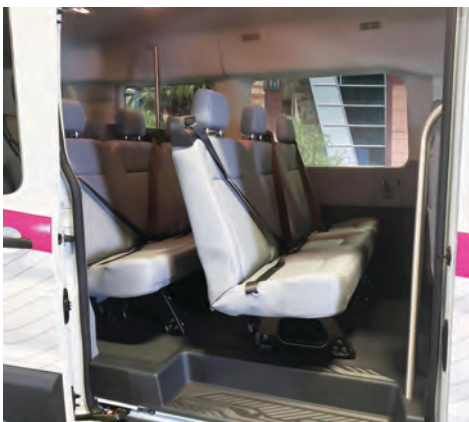
A large step-well and stanchion grab pole provide for easy access to a spacious seating area.
