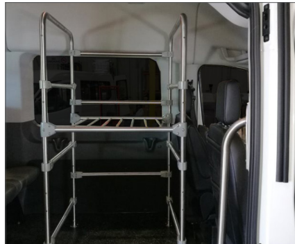
Faster and easier loading and unloading with entranceway handrail and two-tier luggage rack
