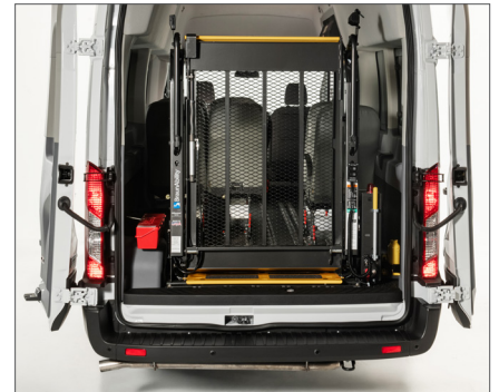
ADA-compliant rear lift with 800-pound capacity
