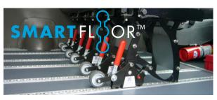
Our exclusive SmartFloor system allows for seats to quickly be removed or changed to create a different seating configuration.
