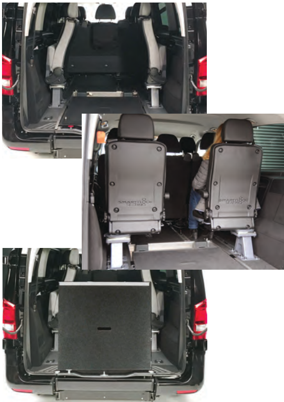
Top: ramp in flat cargo position with third row seats stowed.
