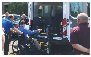
Drivers take turns with using a wheelchair lift and learning the proper procedures for loading and securing a wheelchair passenger. Hands-on training helps to prepare drivers for real-life conditions they will encounter with actual passengers.
