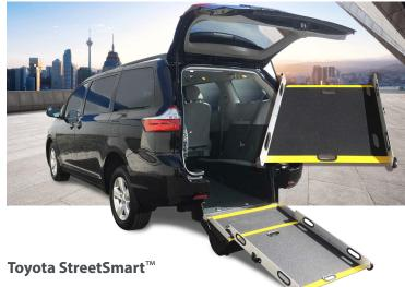
Our patent pending design allows for a removable ramp to be stowed upright – or flat on the floor. It can also be used outside of the vehicle to help with assisting wheelchair passengers navigate over curbs.
